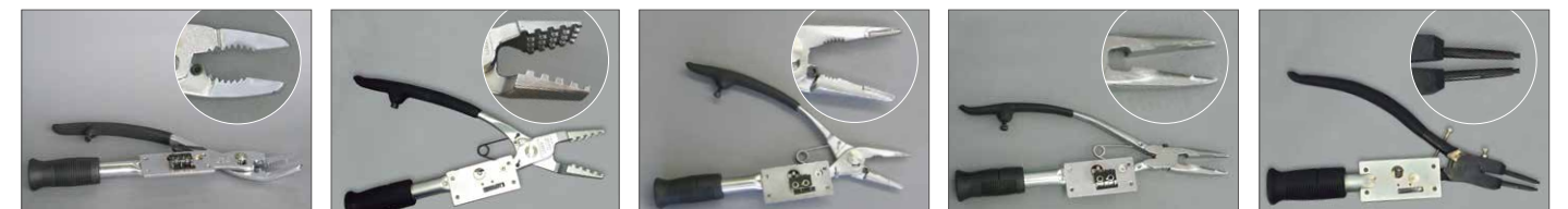
Bent Nose Upward Type [ BN200YU2 ] Length 250 mm (9.8") Weight 410 g (14.5 oz) Jaw Opening 10-12 mm (0.4-0.5") Max. Jaw Opening approx. 25 mm (1.0") Spring Hose Clip Type [ AE-200 ] Length 250 mm (9.8") Weight 500 g (17.6 oz) Jaw Opening approx. 33 mm (1.3") Max. Jaw Opening approx. 33 mm (1.3") Super Wide Jaw Opening Type [ LN240SR ] Length 240 mm (9.4") Weight 350 g (12.3 oz) Jaw Opening 17-20 mm (0.7-0.8") Max. Jaw Opening 30 mm (1.2") Wider Jaw Opening Type [ T-308R ] Length 255 mm (10.0") Weight 380 g (13.4 oz) Jaw Opening approx. 17 mm (0.7") Max. Jaw Opening approx. 17 mm (0.7") Snap Ring (for Shaft) Type [ FOS-185 ] Length 205 mm (8.1") Weight 300 g (10.6 oz) Jaw Opening approx. 6-8 mm (0.2-0.3") Max. Jaw Opening approx. 21 mm (0.8") Use Range of Snap Ring: 10-40 mm (0.4-1.6") Note: There is no function for preventing a false transmission. * Snap ring (for bore) type is also available.
