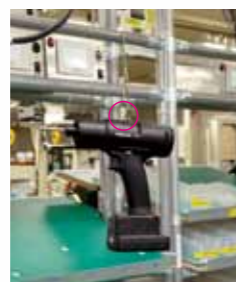
Quickly set the torque by adjusting the scale
