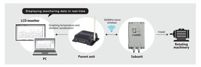
Subunit sensors measure temperature and vibration acceleration, transmitting data to the main unit wirelessly using the 920MHz band.
